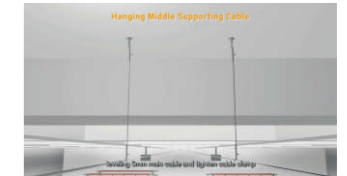
Installation of hanging points
