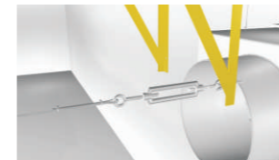
Cable measurement & cutting and connection with bracket
